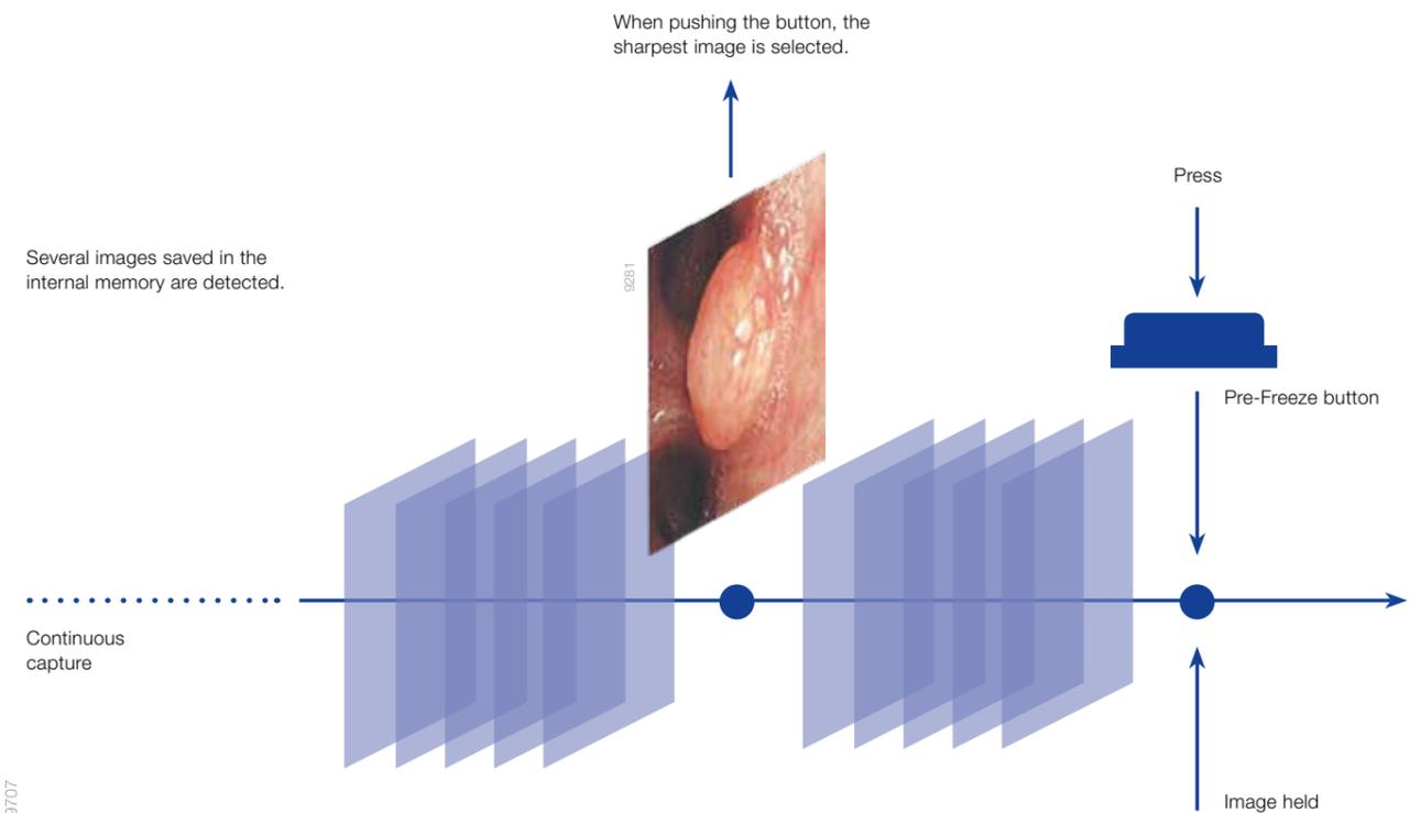
The system continuously buffers a series of images. When you take an image, it automatically analyzes the previous pictures and selects the sharpest one.
